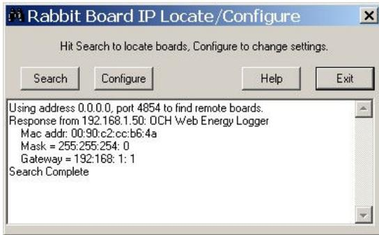
In the example, you can see that the program got a “Response from 192.168.1.50”. This is the WEL’s IP address. You’ll also note that the Gateway address is 192.168.1.1, this is typical for many network routers (like Linksys). If need be, these addresses can be changed by clicking the “Configure” button and entering the desired addresses.
