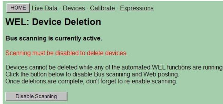
If you are ready to delete devices, click the **Disable Scanning** button. The WEL will be immediately put in idle mode and shortly thereafter; the BUS Status-Bubble on the WEL will start blinking rapidly. This is a visual reminder that you are no longer posting data, and that you should re-enable scanning as quickly as possible.
