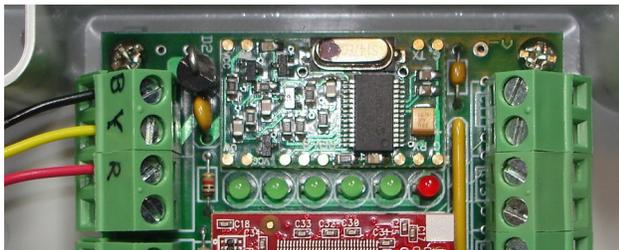
Here you see the Bus cable connected to the WEL using the standard color code.
