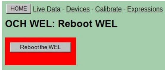
Once a reboot has been requested, the program won't restart for 10-12 seconds until the boot sequence is complete. At that time you may need to use **LocateIP.exe** again if the WEL is assigned a new IP address.
