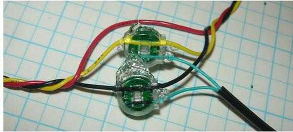
In some situations, it's just not convenient to have one single long bus for all the sensors. In these cases, one incoming pair might need to branch out to several sensors throughout the house (eg: at thermostat locations). Here, the various pairs are connected in "parallel" to form a "Star" network. You MUST limit the number of stars in your system by deciding on a central hub location and only fanning out from there.
